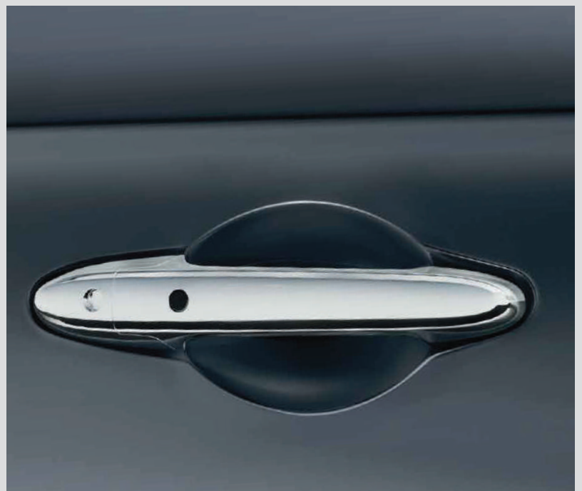
CHROME DOOR HANDLES WITH TOUCH SENSOR BASED SMART ENTRY SYSTEM
