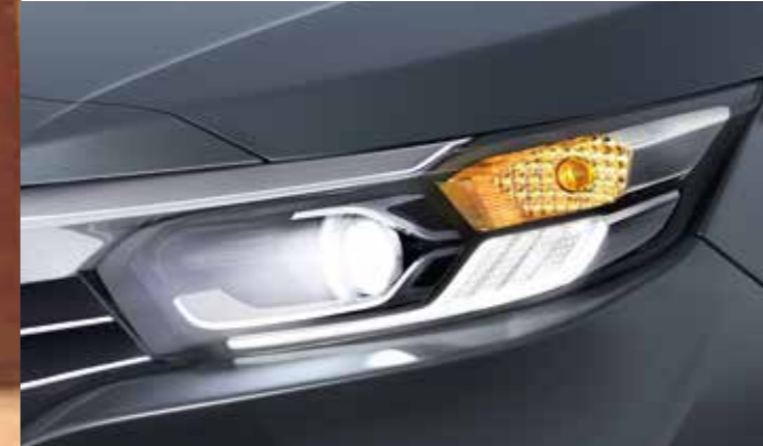
ADVANCED LED PROJECTOR HEADLAMPS WITH INTEGRATED SIGNATURE LED DRLs
