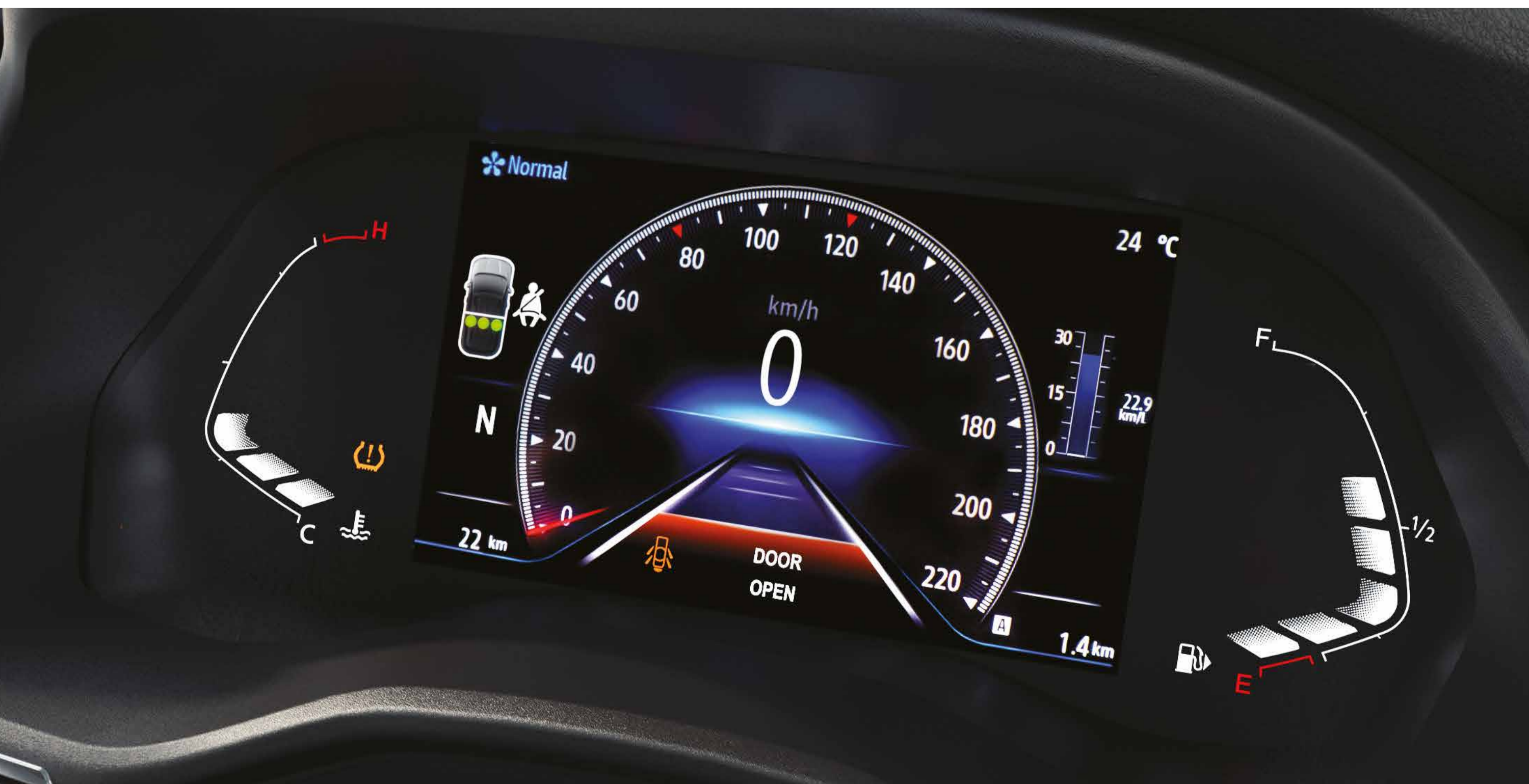
17.78 cm reconfigurable TFT cluster
